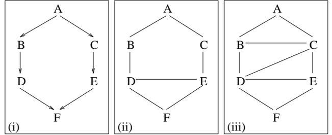
Figure 1: (i) A BN  $\mathcal{D}$ . (ii) The moralization  $\mathcal{U}_m$  of  $\mathcal{D}$ . (iii) One possible triangulation  $\mathcal{U}_t$  of  $\mathcal{U}_m$ . The MN defined by the maximal cliques of  $\mathcal{U}_t$  is  $\mathcal{H} = \{ABC, BCD, CDE, DEF\}$ .
